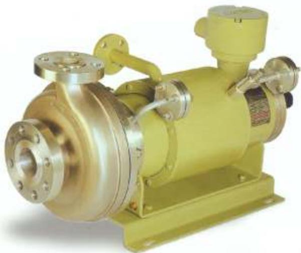
TYPE HT pumps are designed for high temperature fluids up to 400°C. The pump and motor are separated thermally by an adaptor which prevents heat transfer from the pump to motor area. In these pumps an independent circulating system with cooling jacket and heat exchanger is provided. The circulation is achieved with the aid of an auxiliary impeller mounted at the fore end of the motor chamber.
