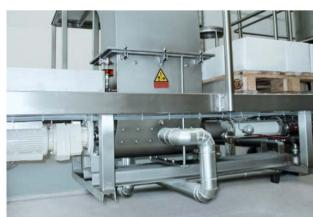
Pump of range BTM 10-12 Conveying product: Various fruits Conveying capacity: max. 7 m<sup>3</sup>/h (31 GPM) • Pressure: 12 bar (174 PSI) Temperature: 10–20 °C (50–68 °F)
