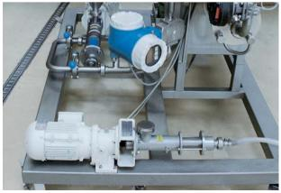
Pump of range MD 006-12 Conveying product: Blancmange Conveying capacity: max. 120 l/h (0.5 GPM) • Pressure: 4 bar (58 PSI) Temperature: 20 °C (68 °F)
