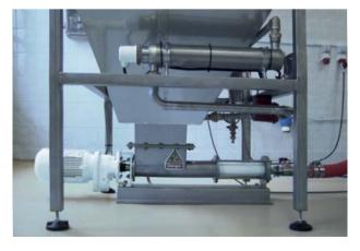
Pump of range BTCS 1-12 Conveying product: Fruit mass Conveying capacity: max. 380 l/h (1.6 GPM) • Pressure: 6 bar (87 PSI) Temperature: 5–40 °C (41–104 °F)
