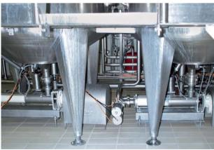
Pump of range BCSO 17-6L Conveying product: Curd-fruit mixture Conveying capacity: 3.5–16 m<sup>3</sup>/h (15–70 GPM) • Pressure: 4 bar (58 PSI) Temperature: 5–20 °C (41–68 °F)
