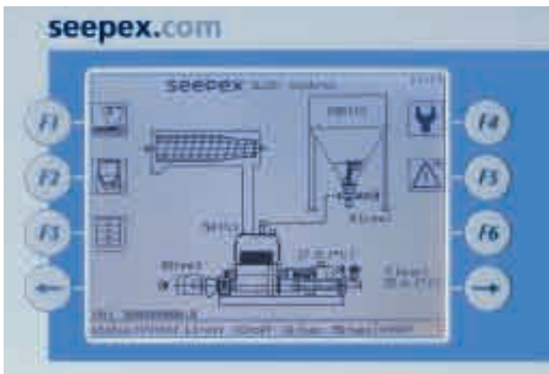
Display of control SLCO for monitoring of the complete process
