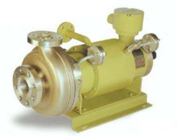
TYPE HT pumps are designed for high temperature fluids up to 400°C. The pump and motor are separated thermally by an adaptor which prevents heat transfer from the pump to motor area. In these pumps an independent circulating system with cooling jacket and heat exchanger is provided. The circulation is achieved with the aid of an auxiliary impeller mounted at the fore end of the motor chamber.
