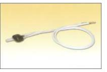
of the cooling system. As a precaution from damage of the motor a thermostat is embedded in the hot spot of the winding to protect the motor from over heating. Thermostat is usually of the closed contact type which will open out at the precautionary preset temperature causing the motor protection circuit to trip off the motor. Thermostats are installed with the motor of Canned Motor Pump, as a standard feature.
