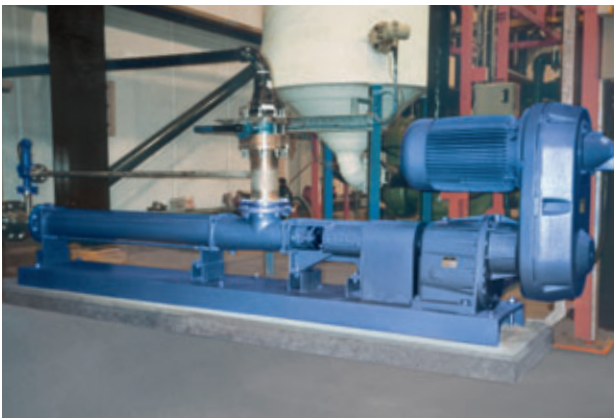
Pump of range NS 70-18 Conveying product: Oily water Conveying capacity: 50 m 3 /h (220 GPM) • Pressure: 15 bar (217 PSI) Temperature: 55 °C (131 °F)
