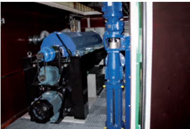
Pump of range BN 35-6LS Conveying product: Oil based drilling mud Conveying capacity: 20 m 3 /h (88 GPM) • Pressure: 3.5 bar (50 PSI) Temperature: 30 °C (68 °F)
