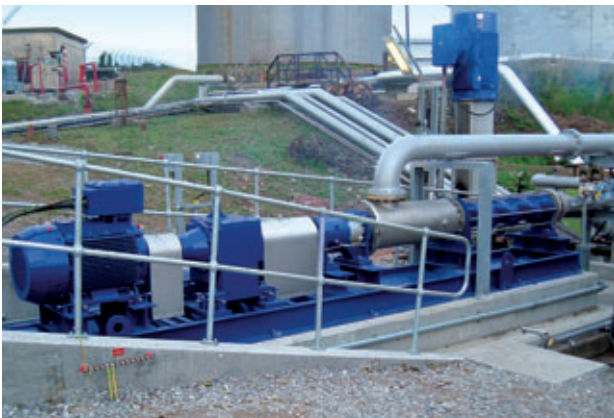
Pump of range N 240-12V Conveying product: Crude oil Conveying capacity: 150 m 3 /h (660 GPM) • Pressure: 19 bar (275 PSI) Temperature: 5–40 °C (41–104 °F)
