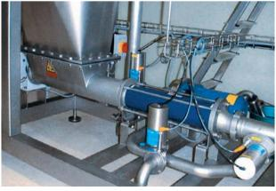
Pump of range BTCS 10-12 Conveying product: Tomato paste Conveying capacity: 1.3 m³/h (6 GPM) • Pressure: 4 bar (58 PSI) Temperature: 10–20 °C (50–68 °F)
