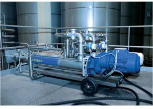
Pump of range BCSB 35-6L Conveying product: Wine Conveying capacity: 32 m³/h (140 GPM) Pressure: 2 bar (29 PSI) • Temperature: 20 °C (68 °F)
